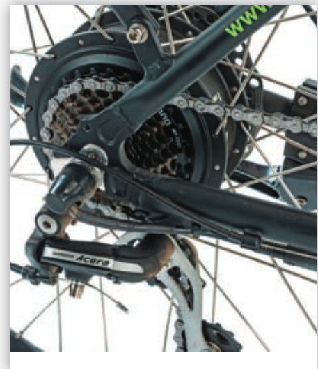
The Shimano seven-speed cassette shifted true, but we found we ran out of gears easily on flat ground.
