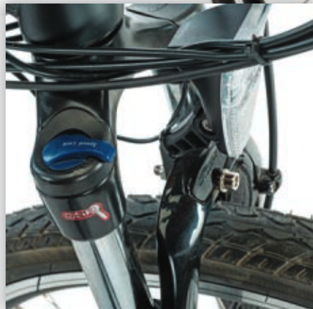
The SR Suntour NEX fork is e-bike-specific and provided enough travel to dampen every bump we found. We never used the built-in lockout.
